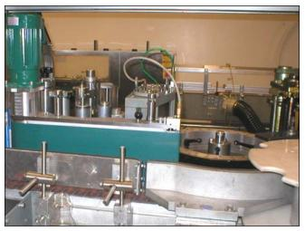
The Discharge Stabilizer System controls unstable (e.g., empty, tall and thin) containers as they leave the roll-on pad.
