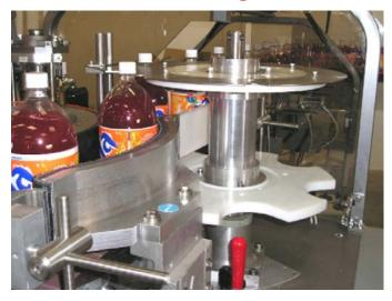
Advanced Change Parts, available on any Trine labeler with a Feedscrew Drive System, include product-specific roll-on pad, vacuum drum, star wheel(s), infeed guides, backing plates and feedscrew.
