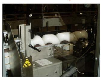
The Feedscrew Drive System is highly recommended for machines operating above 200 cpm, empty and soft bottle applications, and containers that are difficult to handle.
