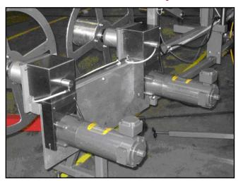
This upgrade provides gentler handling of narrow (< 2 inches), thin (< 35 micron), or easier-to-tear (monolayer film) labels, as well as other labels being applied above 400 cpm.
