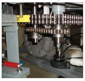
The Dual Chain Drive System upgrade replaces the single #40 chain with double #50 chains on critical drive chains and their related sprockets and chain tensioner.
