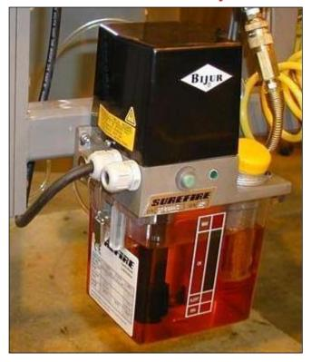
The Automatic Lubrication System upgrade automatically provides lubricating oil to the main drive chains. The amount of lubrication is metered based on total run time of the machine and the setting on the lube pump. This system is electronically controlled, requiring an occasional check of the reservoir.
