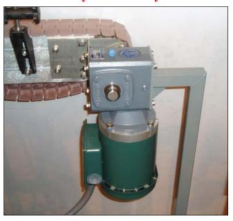
The Conveyor Drive System upgrade replaces the conveyor internal drive chain and delivers more torque directly to the conveyor.
